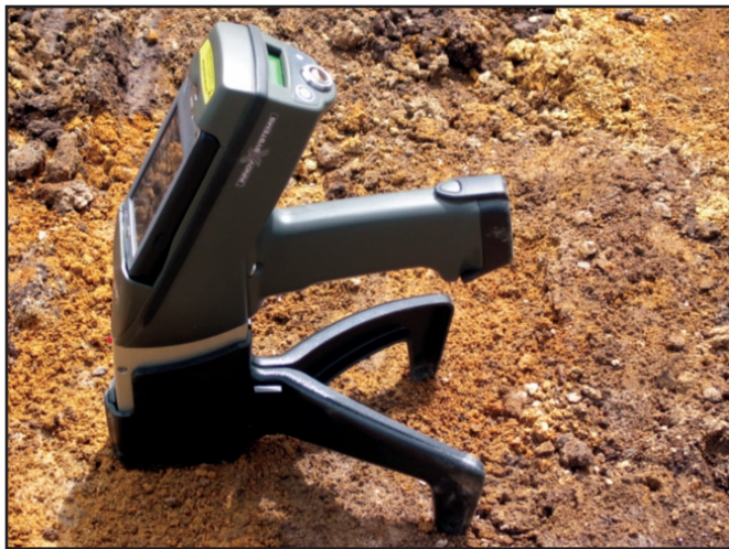
Figure 5—An x-ray tube device being used to check for heavy metals in the soil.
