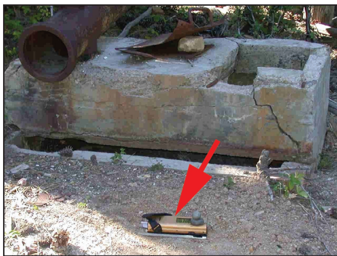
Figure 4—A radioisotope device (arrow) being used to check for heavy metals in the soil.
