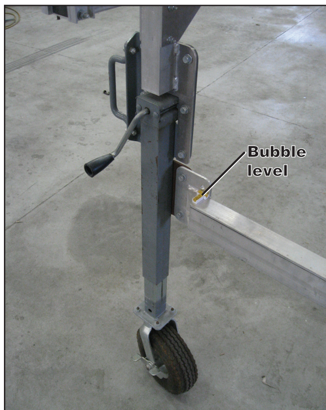
Figure 9—The manual leveling system used in the MTDC prototype top pruner.
