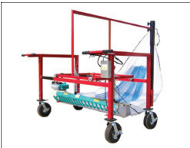
Figure 2a—The EZ Cut Trimmer with a 5-foot, 3-inch-long cutting blade— photo courtesy of AgriNomix.
