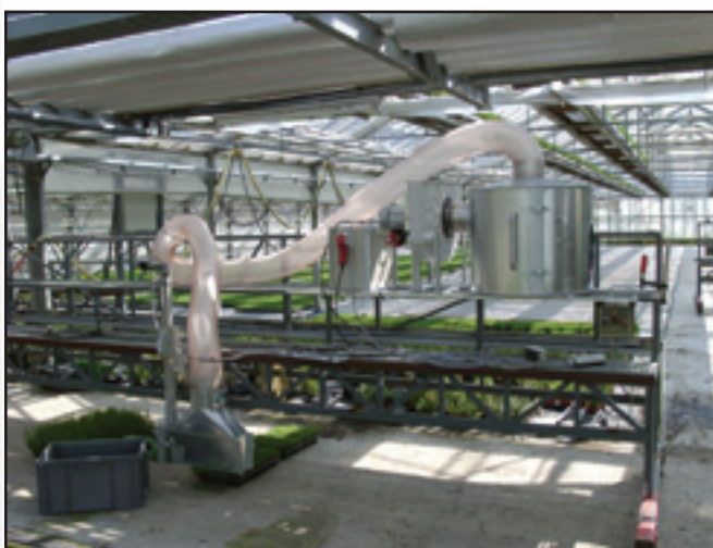
Figure 4—A custom top pruner built with AgriNomix components— photo courtesy of AgriNomix.
