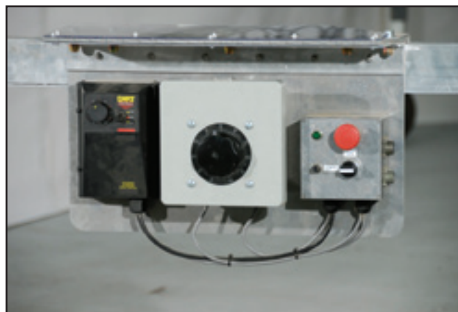
Figure 7—The variable speed control for the cutter and paddle assembly.
