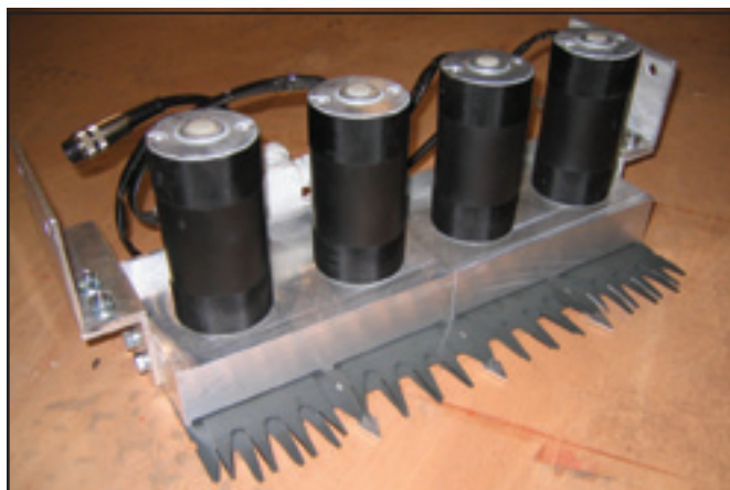
Figure 3c—A precision cutting head with Gardena blades— photo courtesy of AgriNomix.
