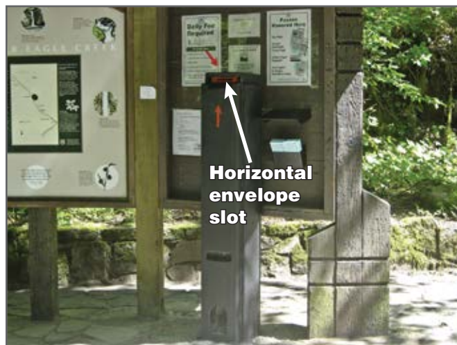
Figure 2—A fee tube with a horizontal envelope slot.
