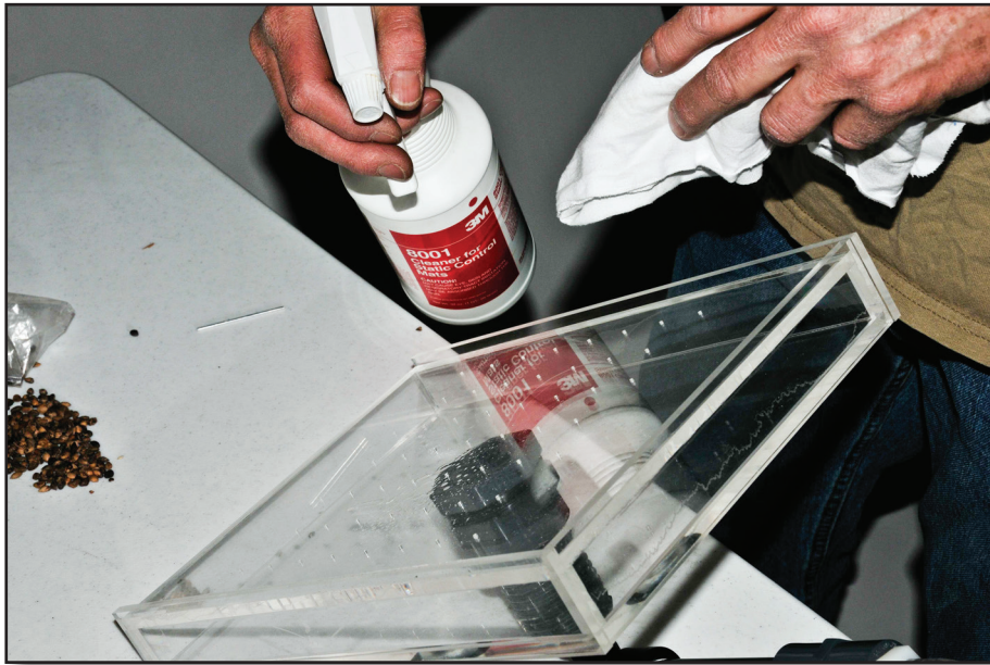
Figure 10—Apply antistatic solution on the acrylic face to prevent seeds from sticking to the pickup head. Fabric softener sheets also may work.
