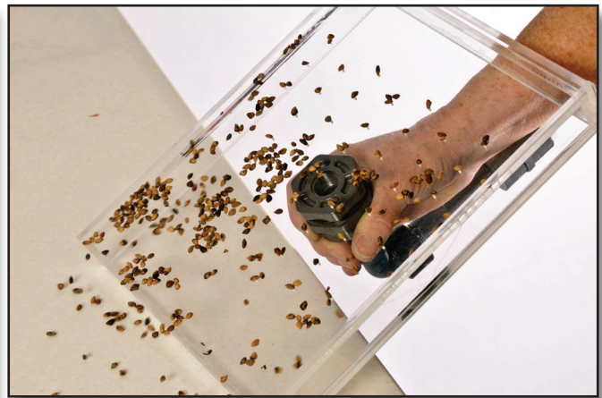
Figure 13—Tilt the pickup head and excess seeds will slide off.
