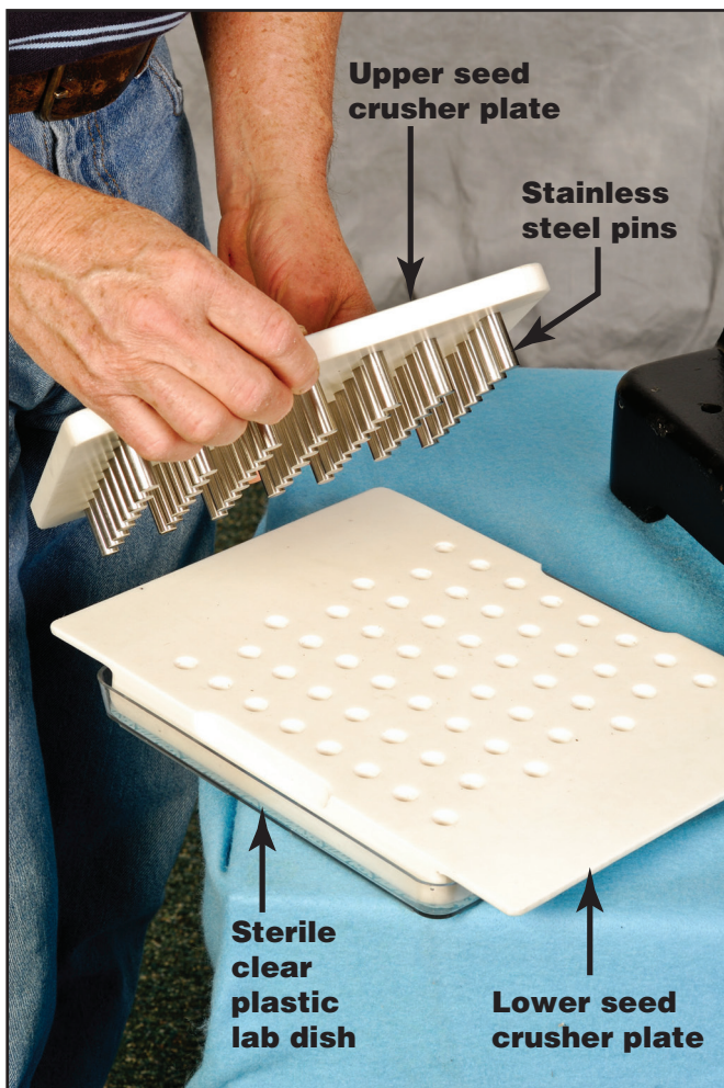
Figure 2—The prototype seed crusher assembly: upper seed crusher plate, stainless steel pins, lower seed crusher plate, and sterile clear plastic lab dish.
