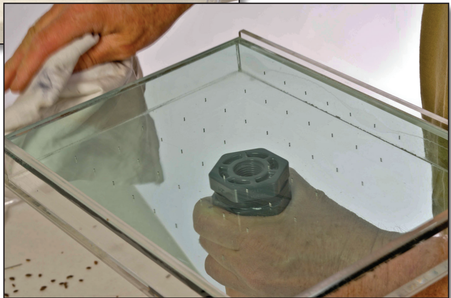
Figure 9—The tinted vacuum pickup head is for smaller pine seeds.
