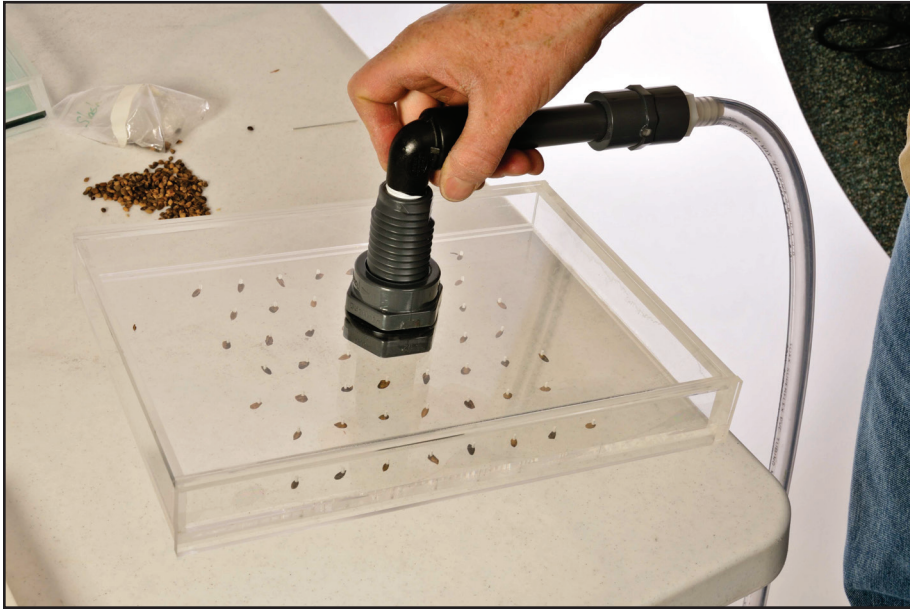
Figure 14—Check seed placement by turning the pickup head over.
