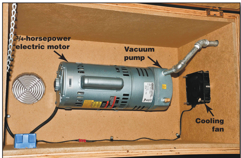
Figure 5—The motor, vacuum pump, and cooling fan are contained in an insulated, sound-dampened box.
