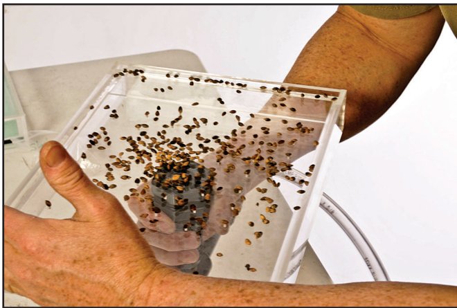
Figure 12—When swirling seeds, cover the side of the pickup head that doesn't have a raised edge.
