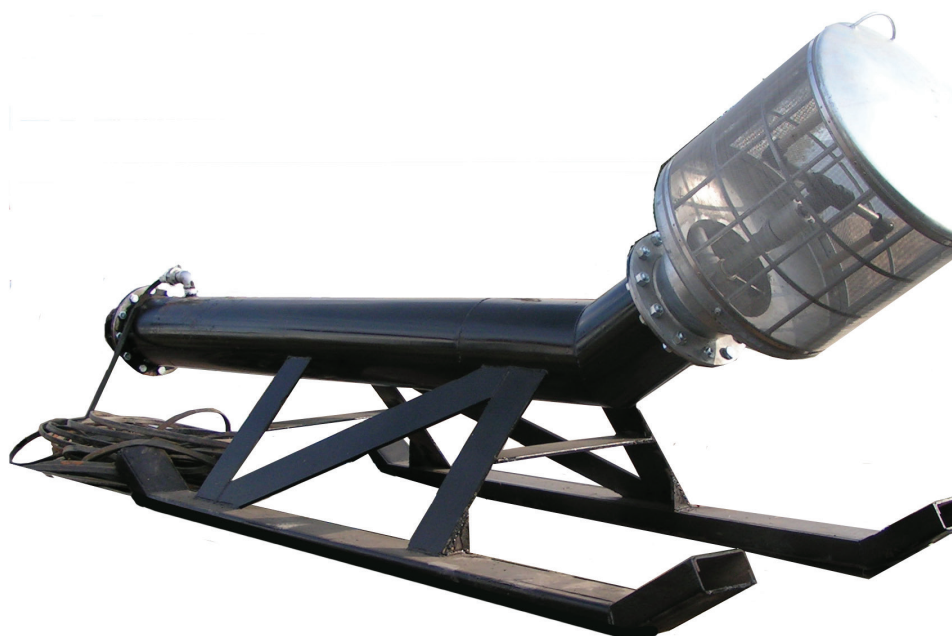
Figure 4.28—Submersible pump on skids to raise it off the streambed. Mounted to the pump housing is a fish screen cleaned by a water-backwash system.
