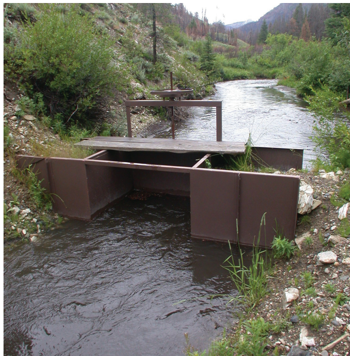
Figure 3.4—Measuring the height of water above the invert of an orifice gate on North Brush Creek, Medicine Bow National Forest, WY.
