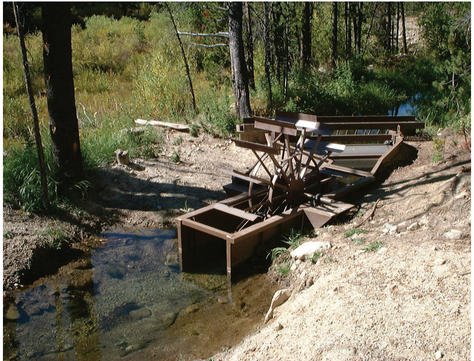
Figure 5.8—Rotary-drum fish screen on Elk Creek, Salmon River Basin, ID. This type of modular setup with a trash-rack and rotary-drum screen powered by a paddlewheel is very common in mountain streams in Idaho and other Western States in anadromous fish habitat.
