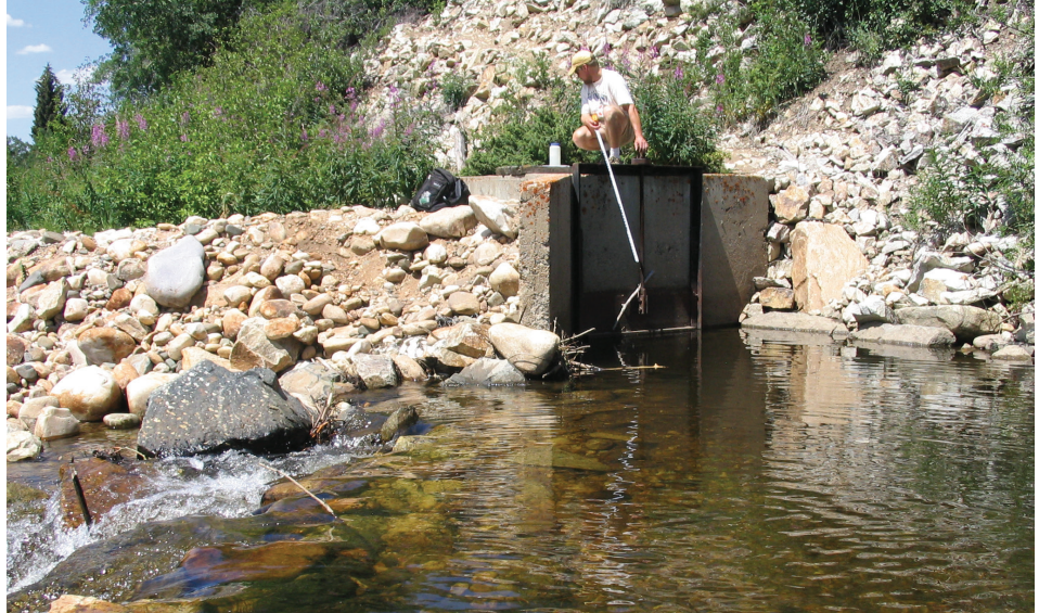
Figure 3.4—Measuring the height of water above the invert of an orifice gate on North Brush Creek, Medicine Bow National Forest, WY.
