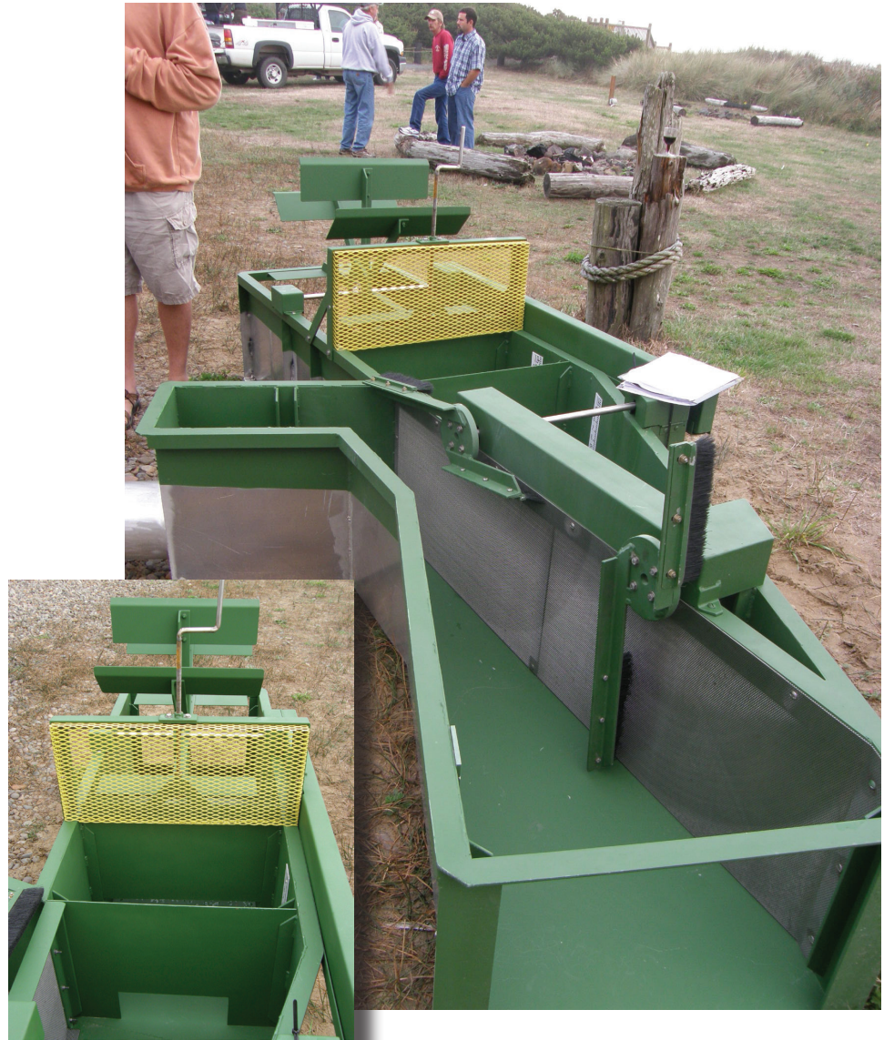
Figure 6.7—A rectangular orifice flow measurement component is designed into this modular vertical flat plate fish screen, designed by Pat Schille, and constructed at the Yakima, WA, screen shop.
