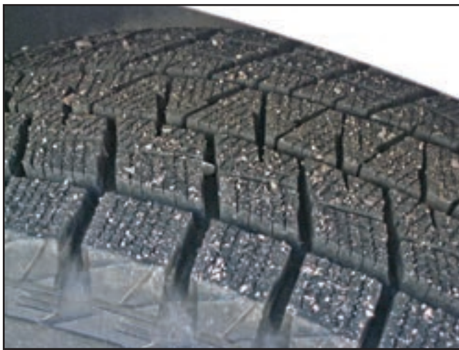
Figure 3—Studless tires employ various techniques to improve traction, such as this Bridgestone Blizzak tire that uses a special rubber compound with microscopic pores.
