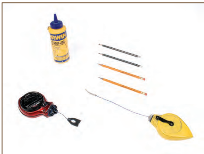
Figure 108—Use pencils and blue chalk (as shown in this photo) on logs, not markers or red chalk. Marker ink and red chalk will not wear off and will bleed through paint and stain. The pencils in the upper right of the photo are blue ink pencils—when you spray the pencil line with water, the line turns blue. Blue lines are easier to see on logs than are graphite lines.
