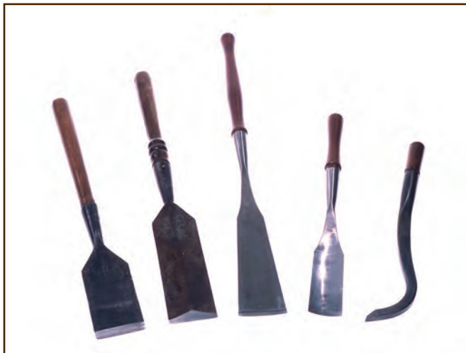
Figure 99—From left to right, these tools are two antique 3 1/2-inch slick chisels, a Barr 3 1/2-inch scarf slick chisel, a Barr 2 1/2-inch gouge, and an antique swan neck chisel.
