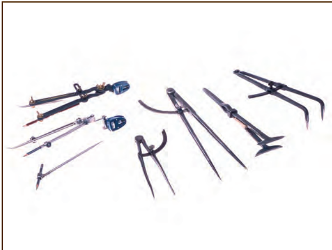
Figure 105—This assortment of scribes includes, counter-clockwise from the left: a Veritas transfer scribe, a Starrett transfer scribe with a separate angled pencil attachment, two old divider scribes, and two different Gränsfors Bruks forged log scribe models.
