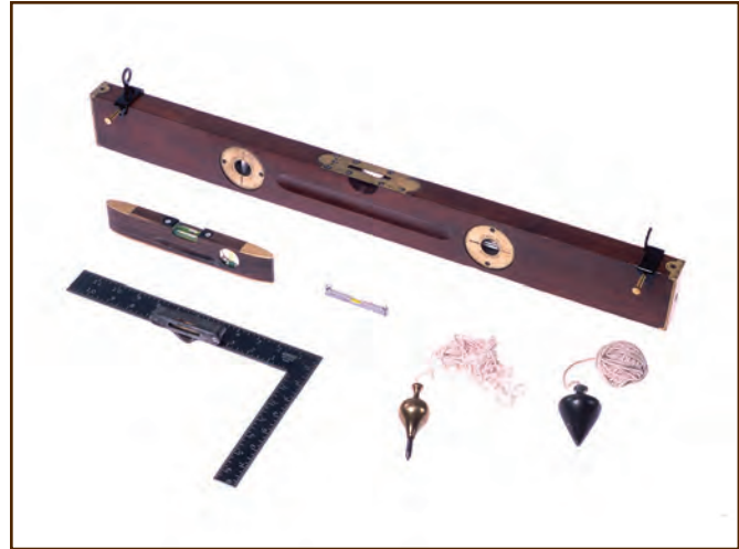
Figure 106—This photo shows some older model plumb bobs and levels, but the newer versions are very similar, although with more plastic parts. Shown are, from top to bottom: a 24-inch-long Stanley wooden level, a wooden torpedo level, a stringline level, a small square with a clamp-on level attached to it, a brass plumb bob, and an iron plumb bob.
