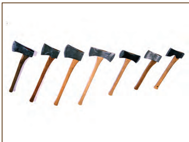
Figure 95—You can find axes and hatchets in a variety of configurations and sizes. This assortment includes, from left to right, a True Temper 5-pound single bit miner's pattern axe with a 28-inch handle, a True Temper 3½-pound single bit Jersey pattern axe with a 32-inch handle, a Hy-Test 6-pound single bit Australian pattern axe with a 32-inch handle, a Bluegrass 3½-pound double bit western pattern axe with a 32-inch handle, a 2½-pound double bit axe with a 24-inch handle, a 2½-pound single bit boy's axe with a 20-inch plumb handle, and a Gränsfors Bruks 1½-pound carpenter's hatchet with an 18-inch handle.
