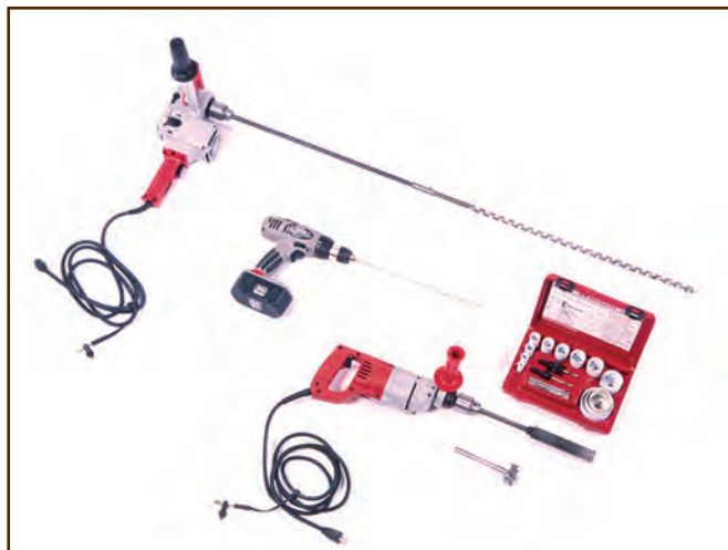
Figure 103—These three tools are, from top to bottom, a Milwaukee Hole Hog with a 24-inch-long, 3/4-inch bit and a 24-inch bit extension; a Porter-Cable 19.2-volt, 1/2-inch chuck cordless drill with a 1/4-inch Irwin bit; and a Milwaukee 1/2-inch hammer drill with a "D" handle and a 1 1/4-inch diamond masonry bit. Also shown are a 2 1/2-inch carbide spur cutter bit and a Milwaukee hole saw kit.
