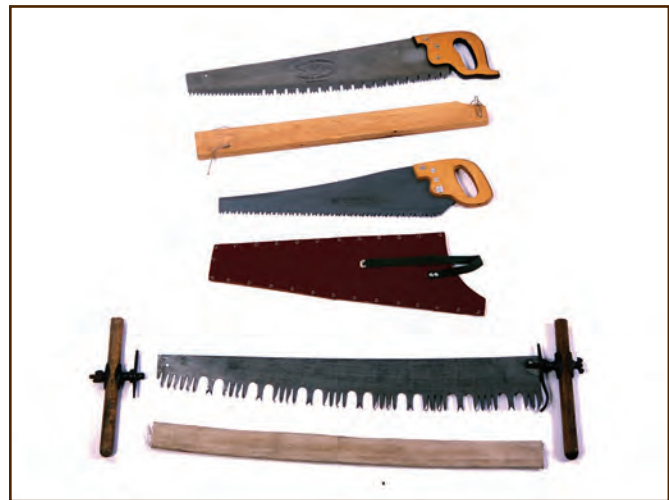
Figure 100—From top to bottom, these saws are a one-man crosscut saw with Great American tooth pattern and its wooden sheath, a Disston champion tooth pattern pruning saw with its leather sheath, and a 4-foot Royal Chinook lance tooth pattern convertible one-man/two-man crosscut saw with its fire hose sheath.
