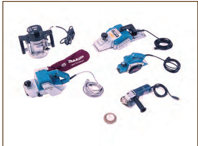
Figure 107—This group of planers, sanders, and grinders includes a 3/4-horsepower, 5-speed Porter-Cable plunge router (top left), a 4-inch Makita belt sander with dust bag (lower left), a 6 1/8-inch Makita planer (upper right), a 3/4-inch Makita planer (middle right), and a Bosch 4 1/2-inch disc grinder with a wood planing disc and a 4 1/2-inch carbide metal wood rasp disc (bottom right).
