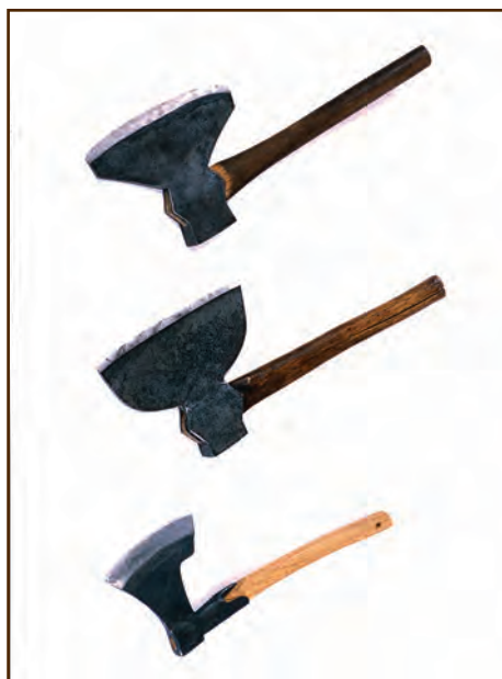
Figure 96—From top to bottom, these three tools are a Gränsfors Bruks 4-pound, 1700 pattern Swedish broad axe with a 17-inch handle; a Beatty 9-pound Pennsylvania pattern broad axe with a 20-inch single bit handle; and a Douglas 8-pound New Orleans pattern broad axe with a 20-inch dog leg (sideways bend) handle.
