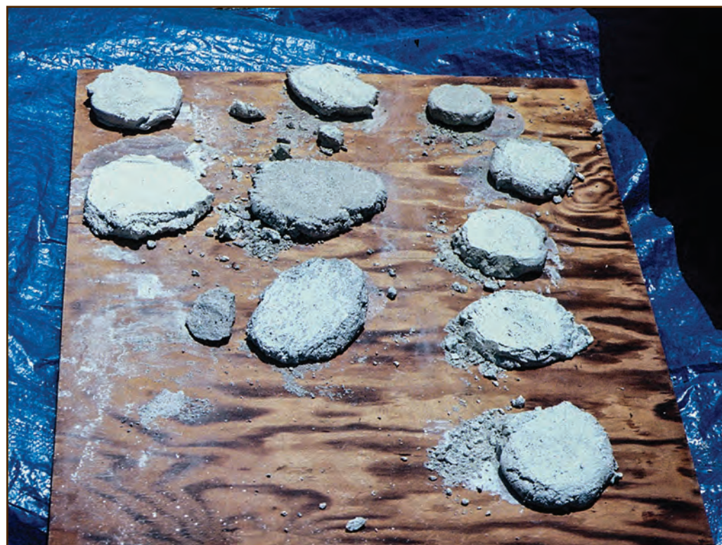
Figure 78—A preservation crewmember shaped several mortar test mixes into patties and allowed them to cure on a plywood sheet. He compared the mixes side-by-side and moved the whole sheet near the original mortared structure to compare them with the original mortar. When you compare mixes, it is easier to see what adjustments you should make to match the original mortar.
