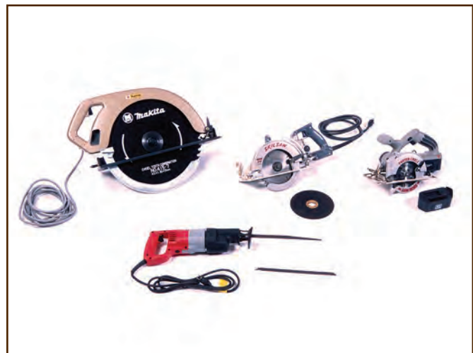
Figure 101—The powertools in the top row are a 16 1/4-inch diameter Makita circular saw, a 7 1/4-inch diameter Skilsaw worm drive circular saw, and a 6-inch diameter Porter-Cable cordless circular saw with an extra battery and battery charger. Below the three circular saws is a Milwaukee Sawzall reciprocating saw with blades for cutting wood and metal.
