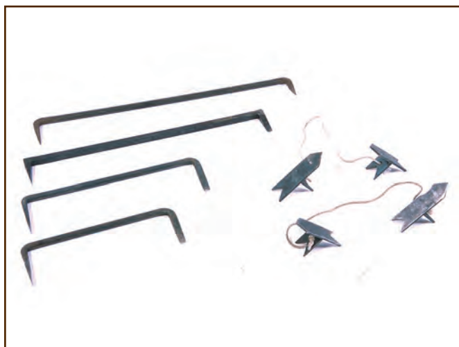
Figure 94—You can find log dogs (on the left, sometimes called log staples) in various sizes with either chisel or pointed ends. The most effective chisel end log dogs are constructed with the flat side on one end perpendicular to the flat side on the other end. Log cleats (on the right) come in pairs connected by ropes.
