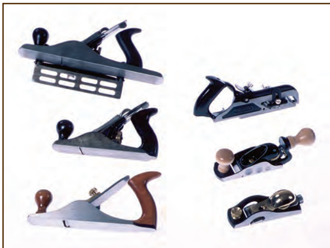
Figure 102—The planes in the left column of this photo are, from top to bottom: an old Stanley #5 corrugated blade jack plane with a plane angle guide, a Lie-Nielsen scrub plane, and a large Veritas low-angle rabbet block plane. On the right, from top to bottom, the planes are: an old Stanley #3 finish plane, a Stanley #78 rabbet plane, and a Lie-Nielsen rabbet block plane.
