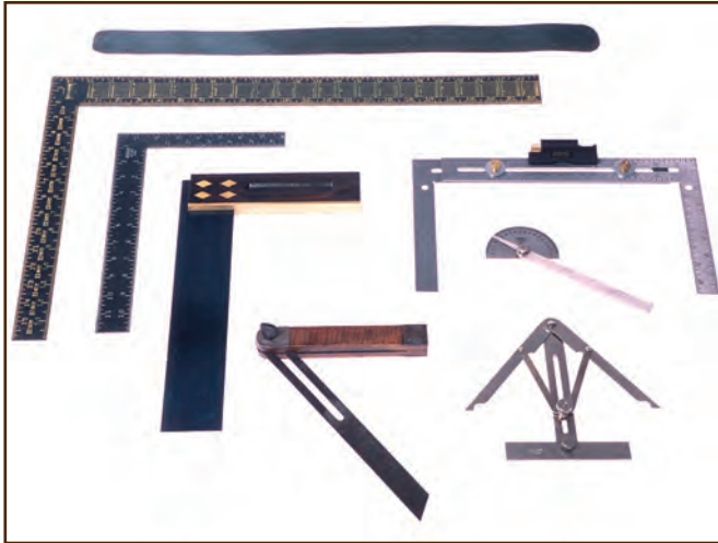
Figure 104—At the top of this photo is a steel band for marking round logs. Other layout and measuring tools on the left are, from top to bottom: a large framing square, a small framing square, a large wood handled tri square, and a sliding “T” bevel. On the right are, from top to bottom: a caliper made from two small squares, a protractor with an extension arm, and an angle divider. A sliding “T” bevel is an adjustable gauge for setting and transferring angles. An angle divider divides the miter angle of inside or outside corners so that trim or other components can be cut properly to fit into odd angles.
