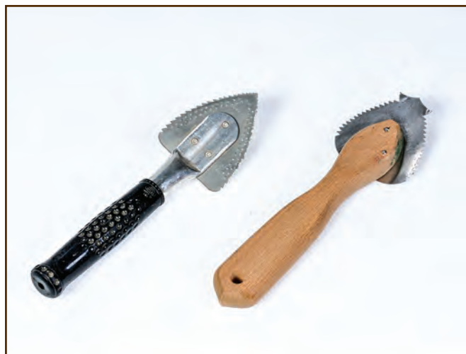
Figure 300—Use window zippers such as these to cut through layers of paint that have sealed a window frame and trim together.
