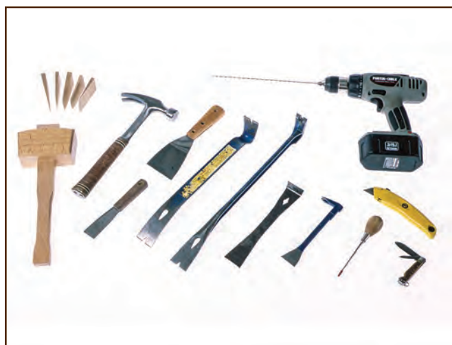
Figure 299—These tools are handy for window work. They are, from left to right, a Woodcraft beech wood mallet and handmade window frame wedges, a smooth-head hammer, two putty knives, three small pry bars, a cat's paw, an awl, a retractable razor blade utility knife, a pocket knife and, at top right, a battery-powered drill with a long bit.
