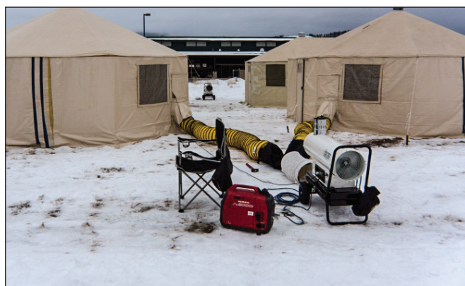
Figure 4—An outdoor propane heater connected to two canvas yurts through flexible ductwork.
