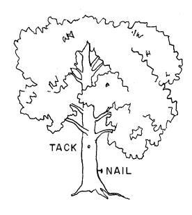
Figure 2. -- Corner tree showing tack and nail.
