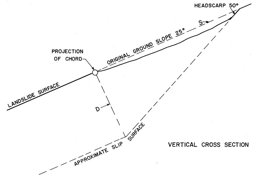
Figure 5. -- Longitudinal Profile of Landslide Slip Surface
