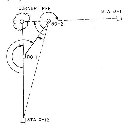
Figure 1. -- Diagram of traverse.
