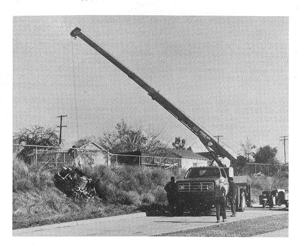
Figure 2. -- Cable crane positioning tree/shrub planter.
