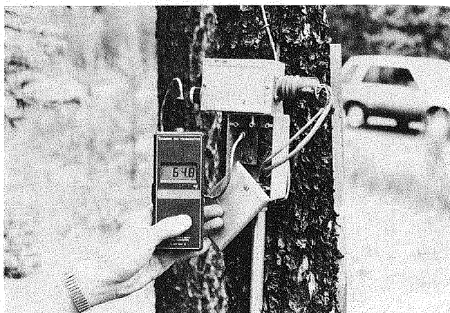
Figure 10.--Electronic thermometer reading the 4-foot sensor (site D2-92-45.2).
