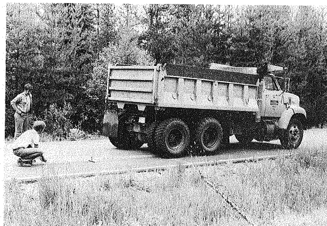
Figure 11.--Benkleman Beam deflection testing (site D2-92-45.2).
