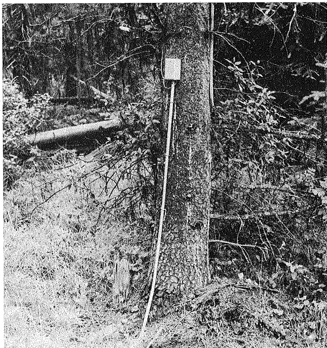
Figure 7.--Junction box, site D-2-92-38.0. Note airprobe on branch slightly above and left of junction box.
