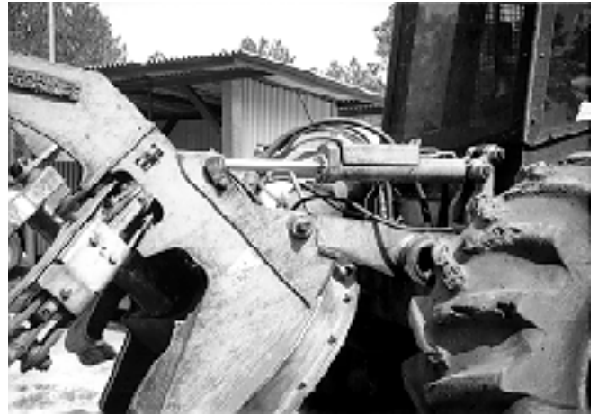
Figure 12a—Operate head through extreme limits of travel to ensure the hose is the proper length and will not get pinched during operation. The head is in the forward position here.
