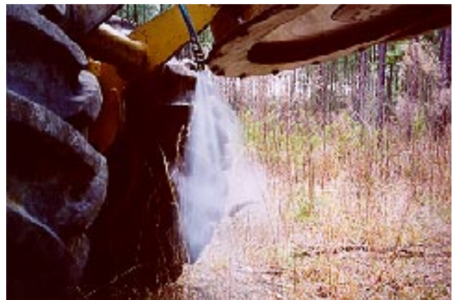
Figure 4—Nozzle at rear of saw head applying powdered borax.
