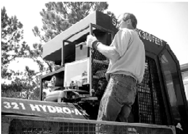
Figure 9—Installing applicator assembly.
