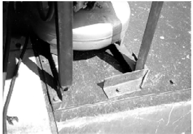
Figure 10—Typical mounting brackets fabricated to attach applicator to existing mounting bolts.
