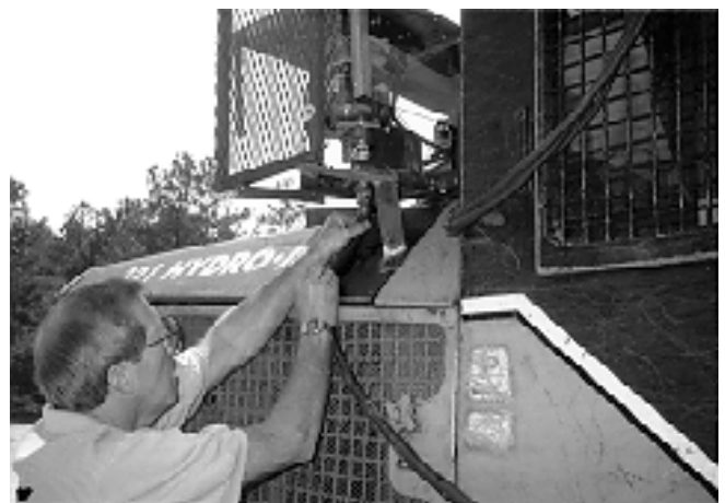
Figure 11a—Route delivery tube from applicator so that it is protected as much as possible without restricting or pinching the tube.
