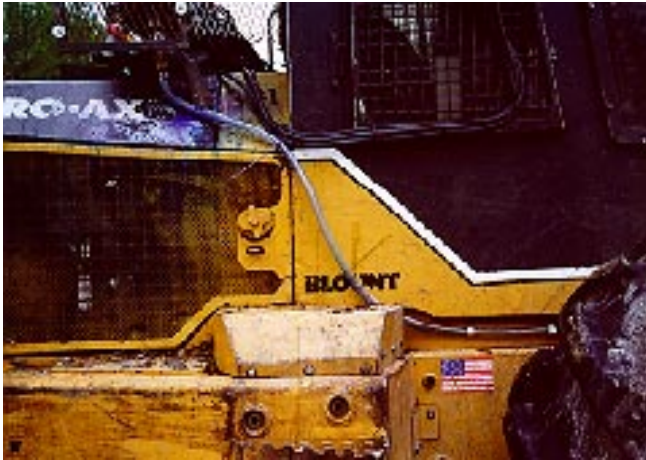
Figure 11b—Use existing machine components to protect the delivery tube.
