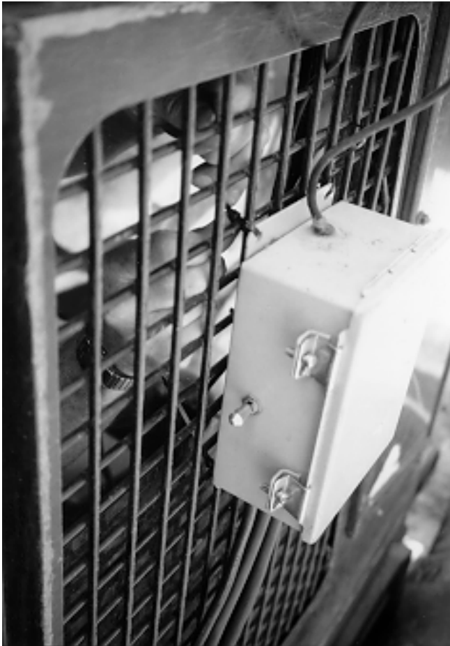
Figure 13—Attaching the electrical control box to the feller-buncher's protective grill.
