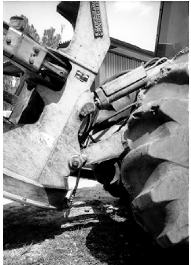
Figure 12b—Operate head through extreme limits of travel to ensure the hose is the proper length and will not get pinched during operation. The head is in the rear position here.
