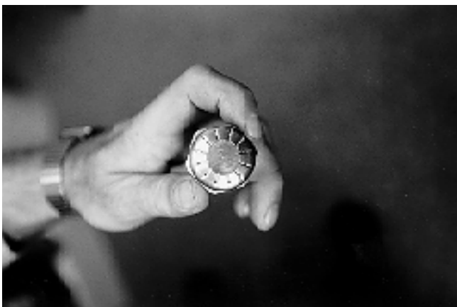
Figure 6—Nozzle with 12 radial delivery holes.
