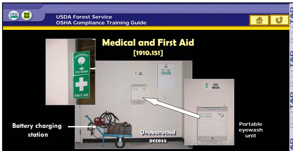
**1910.151(c)** Where the eyes or body of any person may be exposed to injurious corrosive materials, suitable facilities for quick drenching or flushing of the eyes and body shall be provided within the work area for immediate emergency use.
