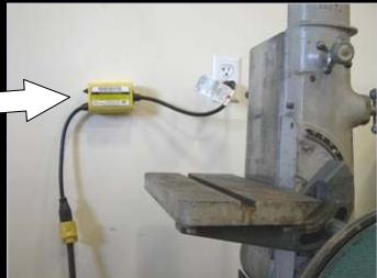
**1910.213(b)(3)** On applications where injury to the operator might result if motors were to restart after power failures, provision shall be made to prevent machines from automatically restarting upon restoration of power.
