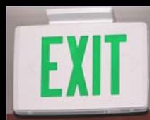
Required exit sign must have plainly legible letters not less than six inches (15.2 cm) high, with the principal strokes of the letters in the word less than three-fourths of an inch (1.9 cm) wide [1910.37(b)(7)]
