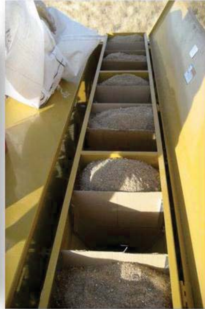
Figure 4. The Truax On-The-Go (OTG) Minimum-till Drill (left); broadcast seed box modification (right).
