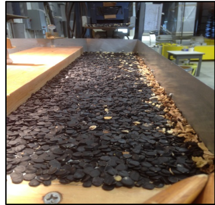
Removing inert material from YUBR on the gravity table. BSE processed more than 1,100 pounds of Yucca spp. during FY14.
